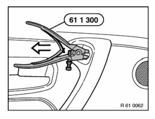
Remove mirror switch with special tool 61 1 300 and pull apart plug connection.
