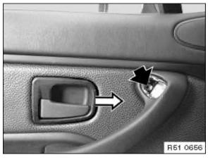
Remove plate forwards. Unscrew screw.
